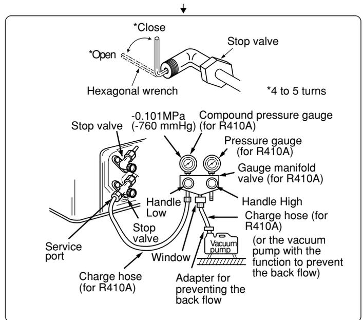
Remove the gage manifold valve quickly from the service port of the stop valve.
